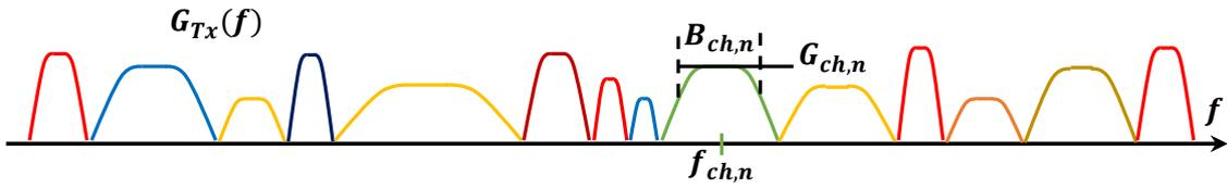
**Fig. 3.1:** Example of possible WDM overall transmission spectrum  $Tx(f)$  having different channels power spectral density,  $G_{ch,n}$  with transmitting lasers at frequencies,  $f_{ch,n}$  and 3dB bandwidth,  $B_{ch,n}$
