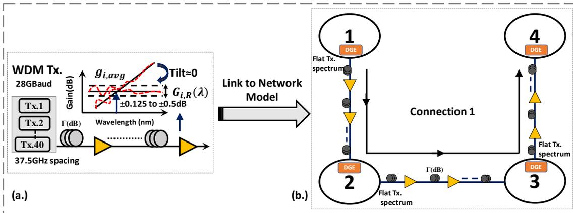
**Fig. 3.4:** Overall migration from (a) STATIC Link Model to, (b) Example of a Network Model
