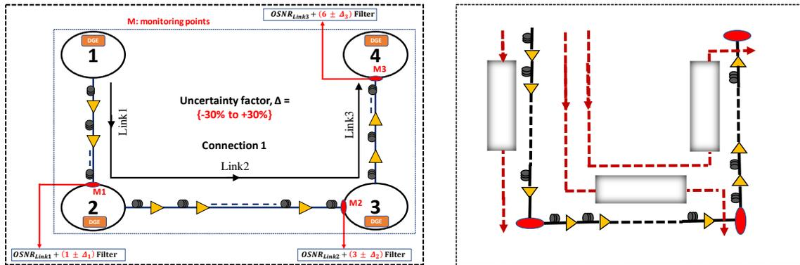
Fig. 4.8: sample connection having filtering uncertainties indicating per (a) link (b) subpath monitoring ports
