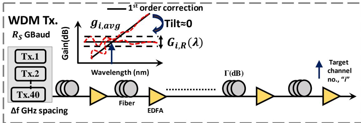
Fig. 3.3: Static link model for span EDFA having Ripple profile
