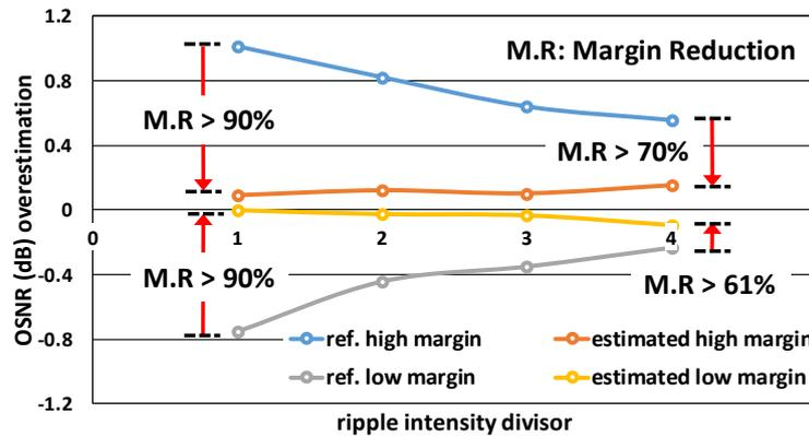
**Fig. 4.6:** New margin for different intensities of peak to peak gain ripple among all EDFAs with reference as  $\pm 0.5$ dB
