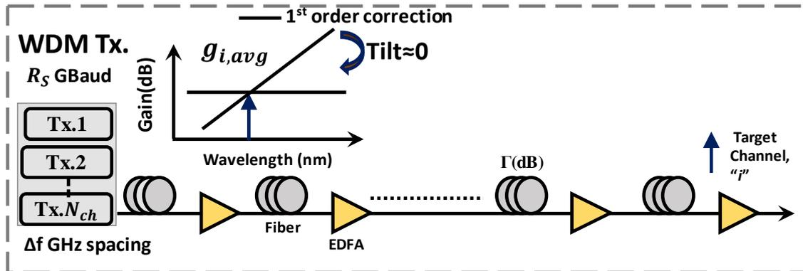
**Fig. 3.2:** Static link model for Flat span EDFA profile
