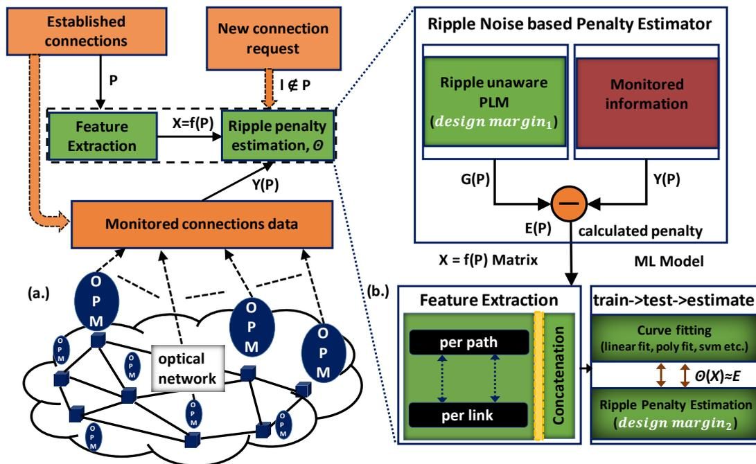
Fig. 4.3: (a) Overall Flowchart and architecture, (b) ML-based penalty estimator (i.e., train/test/estimate)
