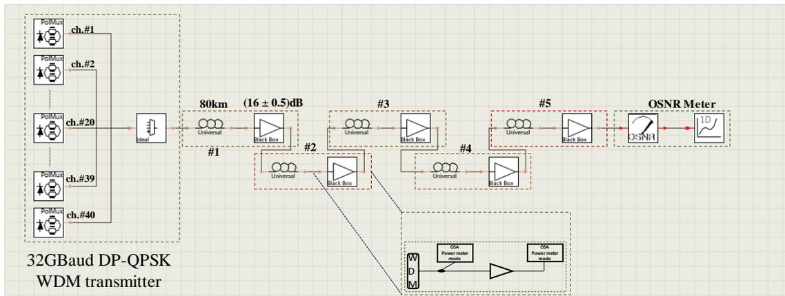
**Fig. 4.1:** VPI Tx. Maker set up for static link having ripple profiles at each span EDFA with peak to peak gain fluctuation,  $g_{i,R}(\lambda) = \pm 0.5\text{dB}$
