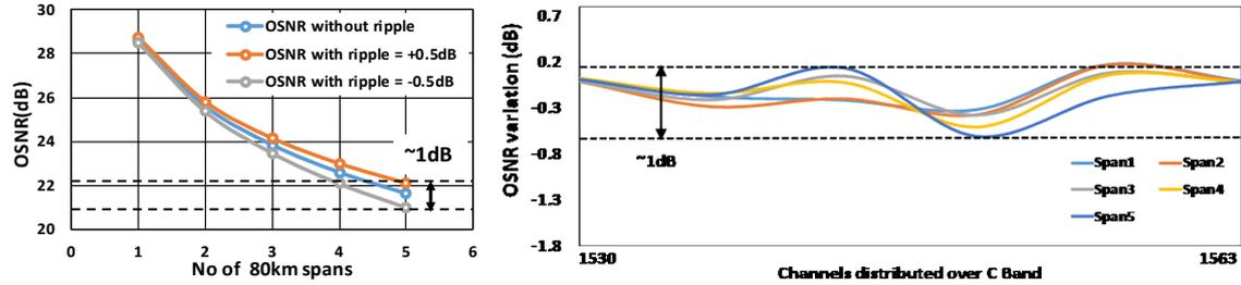
**Fig. 4.2:** (a) OSNR fluctuation of  $\sim 1$ dB observed due to the EDFA gain ripple after 5 spans, (b) EDFA gain ripple effect on OSNR (dB) over the C-band
