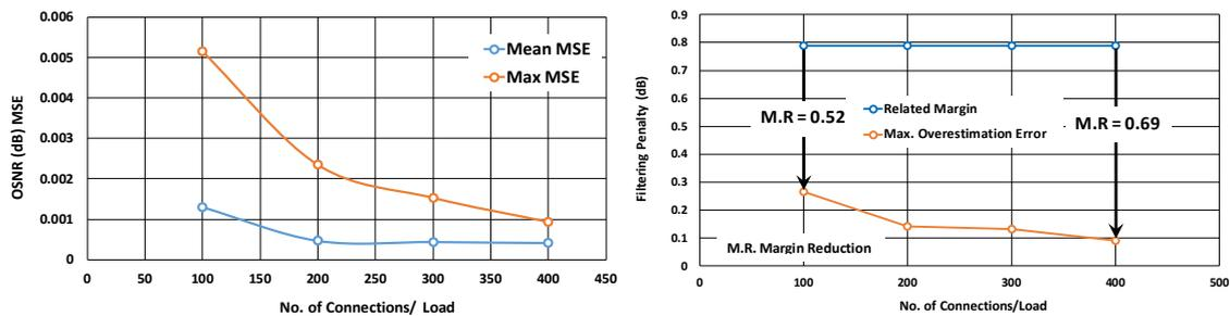
**Fig. 4.9:** Effect of load variation on, (a) OSNR (dB) MSE, (b) Max. overestimation error
