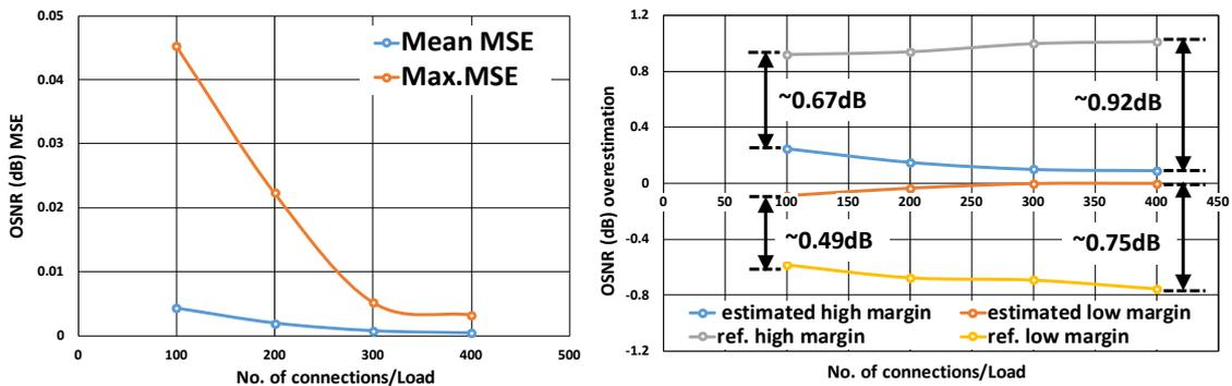
**Fig. 4.5:** Effect of load variation on, (a) OSNR (dB) MSE, (b) Max. overestimation error
