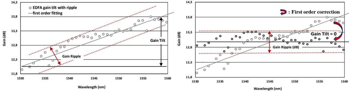
**Fig. 2.1: (a)** Experimentally collected EDFA gain ripple and gain tilt at EDFA output, **(b)** Gain tilt control with zero order / linear correction
