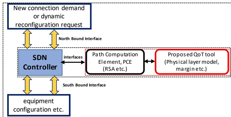
**Fig. 6. 1:** QoT estimation tool interaction with different algorithms
