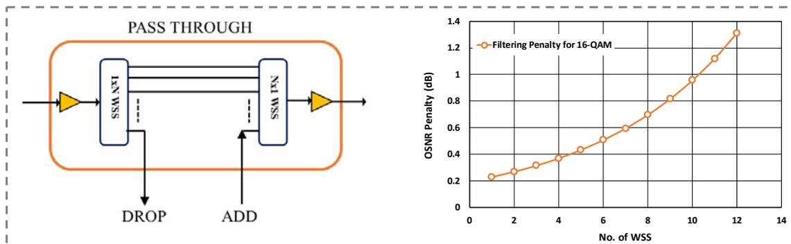
**Fig. 4.7:** (a) A simple switch and select ROADM node architecture, (b) OSNR penalty in dB due to tight optical filtering for 16-QAM
